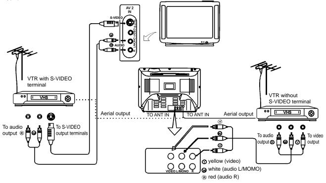
To select the input, press the **TV/AV** button on the TV set or **AV** button on the remote controller repeatedly until you see the corresponding input indication on the screen. To return to aerial input, press the **AV** button until it displays program number, or press channel select button or the CH  $\triangle$ / $\blacksquare$  button.
